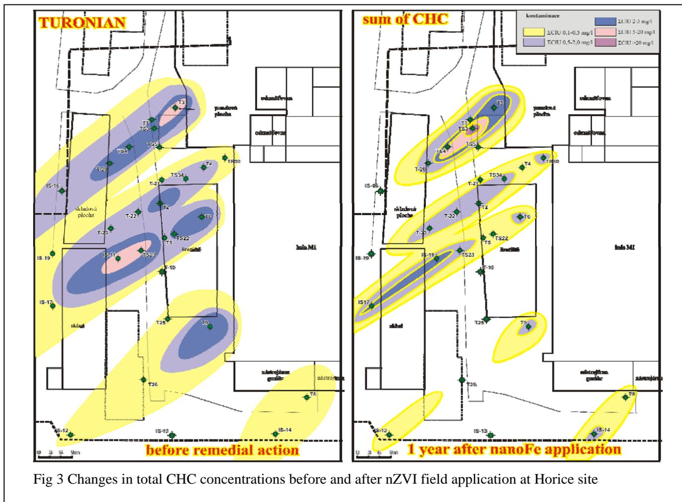
Fig 3 Changes in total CHC concentrations before and after nZVI field application at Horice site
