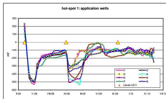
Fig 2 Changes in ORP on the application wells
