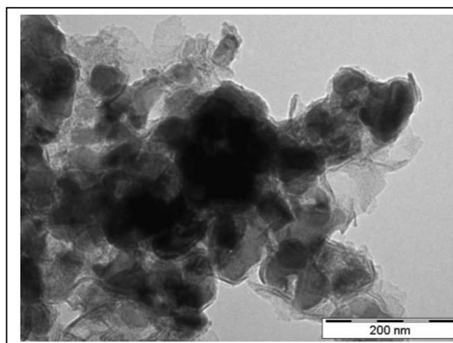
Fig 1 TEM picture of TWEEN80 surface stabilized nZVI
