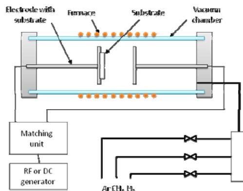
Fig. 1: Schematic diagram of the radio frequency PECVD reactor
