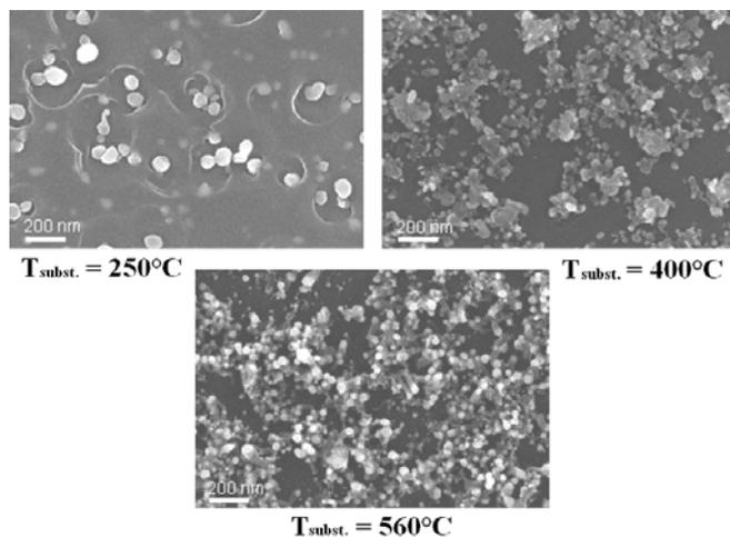
Fig. 2: Surface morphology of samples grown at different substrate temperatures of (a) 250°C, (b) 400°C and (c) 560°C.
