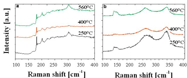
Fig. 3: Raman spectra of samples grown at low, medium and high temperatures: (a) the RBM region and (b) region D and G-bands.
