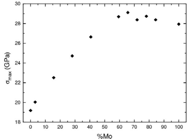
Figure 2: Maximum tensile stress as a function of molybdenum concentration.
