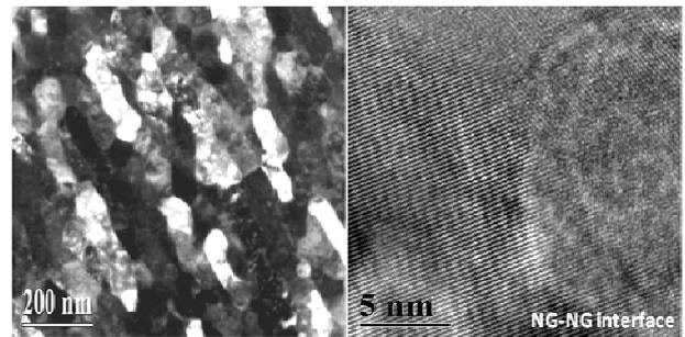
Fig. 6.0 TEM images of deposited AA5083 powder showing mean grain size of  $100 \pm 35 \text{ nm}$  (left) and a grain boundary (right).
