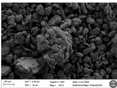
Fig. 1.0: Original n-WERKZ AA5083 feed stock used during the cold spray process. Note large agglomerates.
