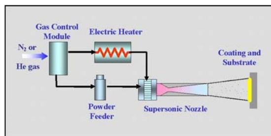
Fig. 3.0: Cold spray system schematic
