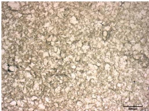
Fig. 5.0 Cold spray deposit of n-WERKZ AA5083. Confocal microscope.
