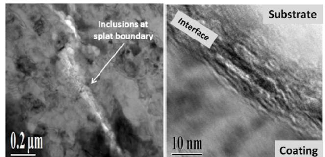
Fig. 7.0 TEM images of grain boundary inclusions (left) and the coating/substrate interface (right).
