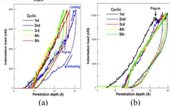
Fig. 3 Load-displacement curves for each indentation cycle on (110) Si at (a)  $P_{\max} = 8000$  nN and (b)  $P_{\max} = 12000$  nN
