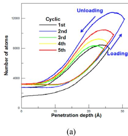
Fig. 2 Variation of total number of transformed atoms in each cyclic indentation cycle on (110) Si at  $P_{\max} = 8000$  nN
