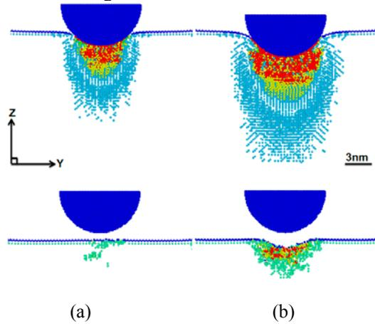
Fig. 1 Side cross-sectional views of the transformation zone and shape of residual indent on (110) Si under the maximum loading (a)  $P_{\max} = 8000$  nN and (b)  $P_{\max} = 12000$  nN after the first indentation cycle.
