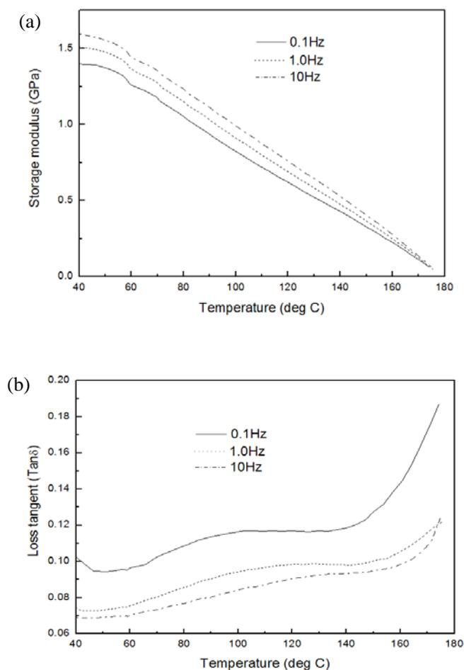
Fig. 3. DMA thermograms of the PP/CNT composites at various frequencies: (a) storage modulus and (b) loss tangent.
