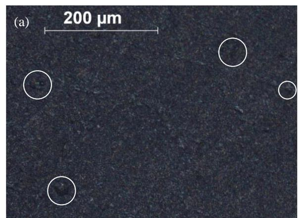
Fig. 2 (a). Optical micrograph of the PP/CNT composite in low magnification,  $\times 100$ . Voids (white circles) are observed inside the sample.
