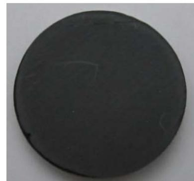
Fig. 1. Photograph of the sintered PP/CNT composite (20 mm in diameter and 3.7 mm in thickness).
