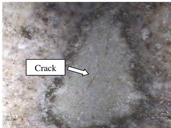
Fig. 3 Polarizing microscope image of H-AN using reactive aggregate after immersion in 1 N NaOH for 28 days at 80°C
