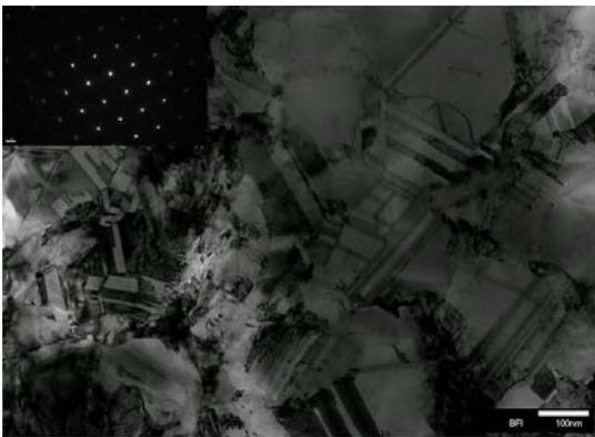
Fig. 2. TEM image and SAD pattern of nickel based iron-zinc composites sheet
