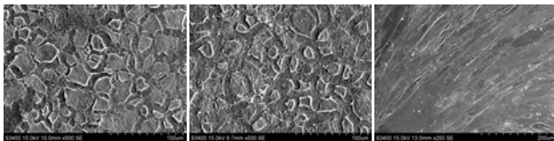
Fig. 2. MSC on nanocomposites with (L-R) 40, 50, and 60% by weight HA at 7 days.
