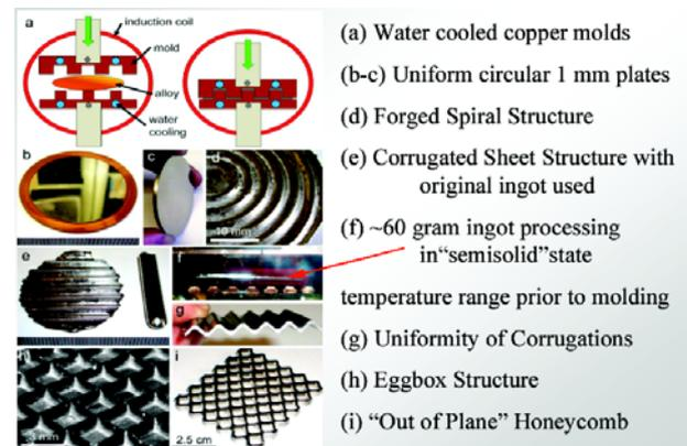
**Figure 1** Wide variety of shapes that can be fabricated using semi-solid processing techniques.
