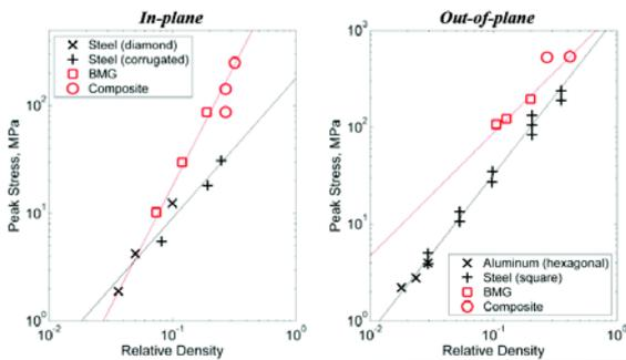
**Figure 3** In-plane (left) and out-of-plane (right) peak load vs. relative density for aluminum, steel, and cellular amorphous [5,6] metals.
