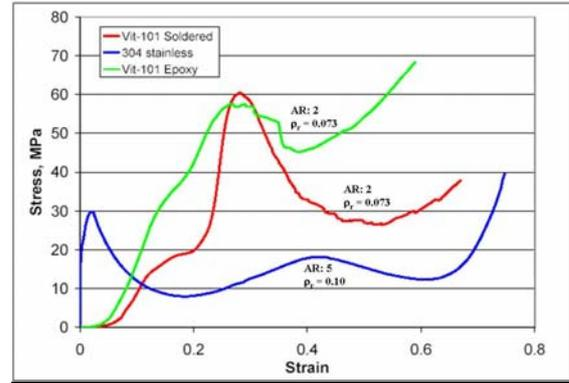
**Figure 5** Out-of-plane stress vs. strain for cellular structures made from Vitreloy 101 ribbon and joined using solder or epoxy, and 304 stainless steel [5].
