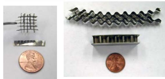
**Figure 2** Out-of-plane cellular structures formed from (left) Vitreloy 101 melt-spun ribbon and (right) corrugated ribbons of Vitreloy 101 and Metglas 2826.
