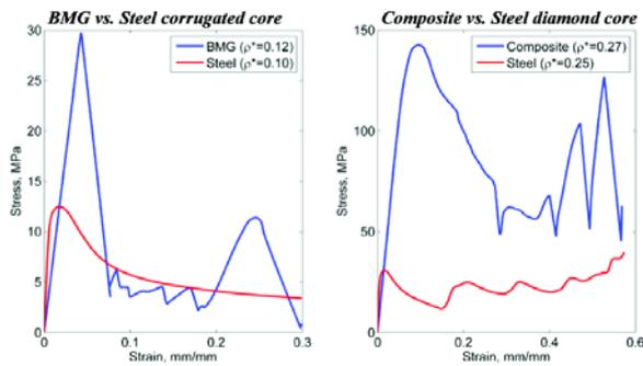
**Figure 4** In-plane cellular composite performance of monolithic BMG (left) and dendritically toughened composite (right) to that of steel [5].
