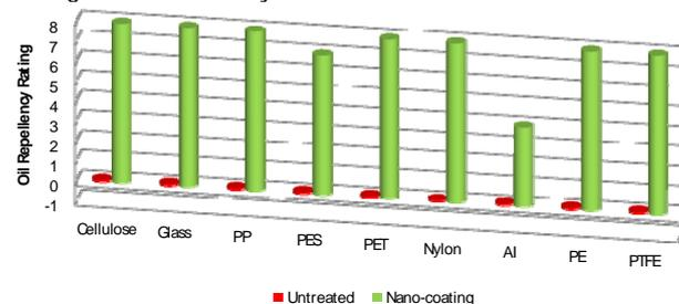
Fig. 2: 3M oil repellency of a variety of uncoated and nano-coated materials
