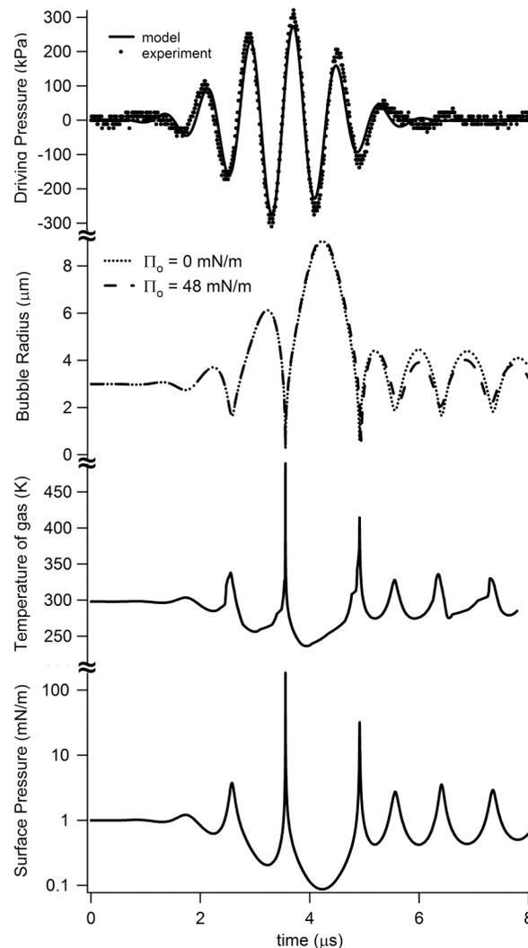
Fig. 2. Numerical solution of the Herring equation.
