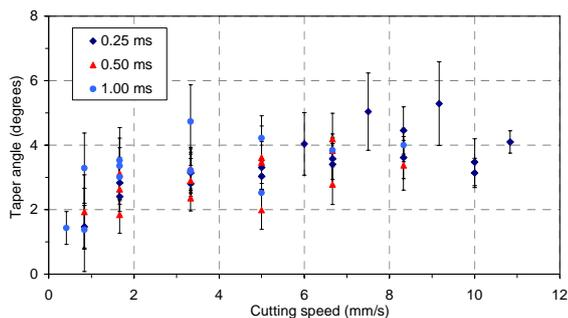
Fig. 4: Taper angle as a function of cutting speed.
