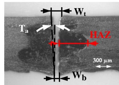
Fig. 1: Kerf section and analysed parameters.
