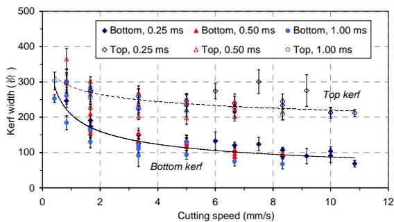
Fig. 3: Bottom kerf width as a function of cutting speed.
