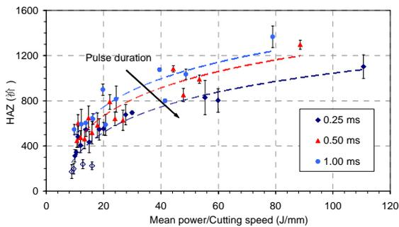
Fig. 2: Influence of the mean power and beam speed on the cutting regions map.
