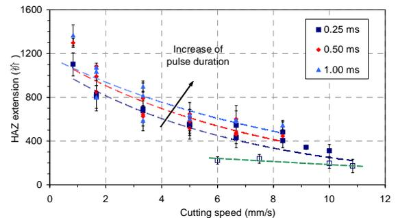
Fig. 5: HAZ extension as a function of cutting speed.
