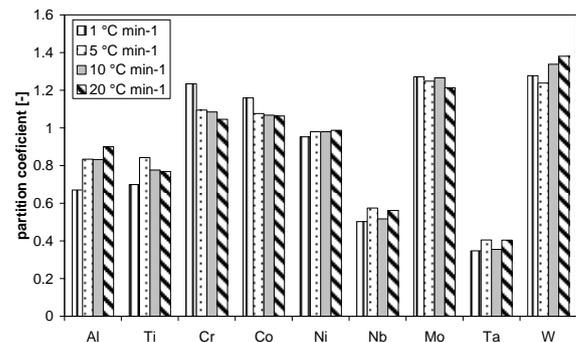
Fig. 4 Ratio of average composition in dendrite cores to interdendritic regions (by EDX) in four samples.
