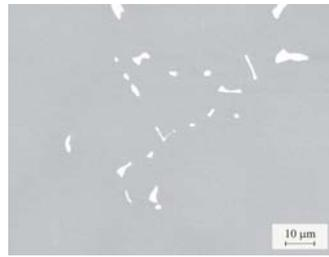
Fig. 3 Morphology of MC carbides, CR 20 °C min<sup>-1</sup>.
