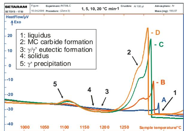
Fig. 1 The DTA curves of samples A, B, C and D.
