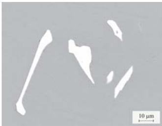
Fig. 2 Morphology of MC carbides, CR 1 °C min<sup>-1</sup>.
