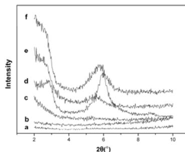
Figure 1. XRD patterns of the different FMMT contents nanocomposites (a) PSAN/FMMT1.5 (b) PSAN/FMMT3 (c) PSAN/FMMT5 (d) FMMT (e) PSAN/FMMT10 (f) PSAN/FMMT15
