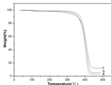
Fig 3. The TGA curves of the products containing different FMMT contents (a) PSAN/FMMT3 (b) PSAN/FMMT5 (c) PSAN/FMMT10
