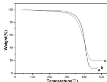
Figure 5. The TGA curves of the products containing different stabilizer contents (a) PSAN/Stab10 (b) PSAN/Stab5 (c) PSAN/Stab0
