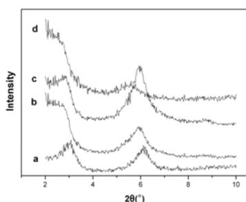
Figure 4. XRD patterns of the different stabilizer contents nanocomposites (a) PSAN/ Stab0 (b) PSAN/ Stab5 (c) FMMT (d) PSAN/ Stab10
