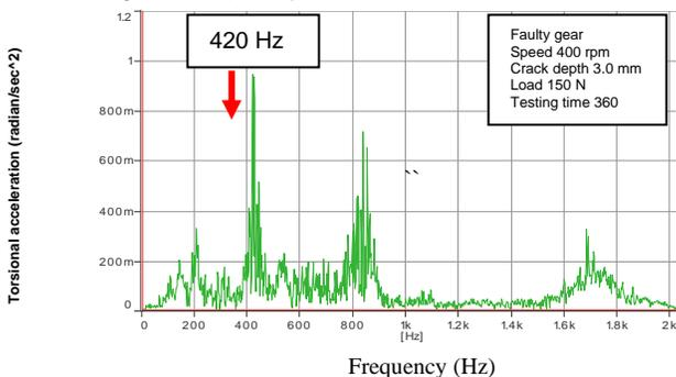
Fig. 2 Frequency-domain torsional
