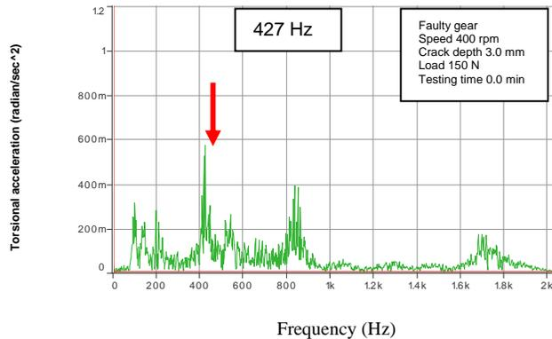
Fig. 1 Frequency-domain torsional acceleration
