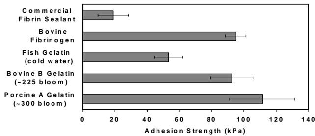
Fig. 2. Adhesive strength of crosslinked materials, comparing photo-crosslinked gelatins with fibrinogen.
