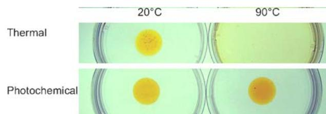
Fig. 1. Thermal stability of crosslinked gelatin.
