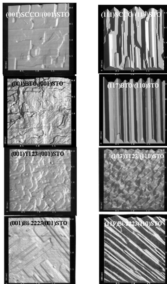
Fig. 3. Atomic Force Microscopy (AFM) images of different films on (001) and (110) STO. Substrates were flat substrates with low miscut angles (typically less than  $1^\circ$ ).
