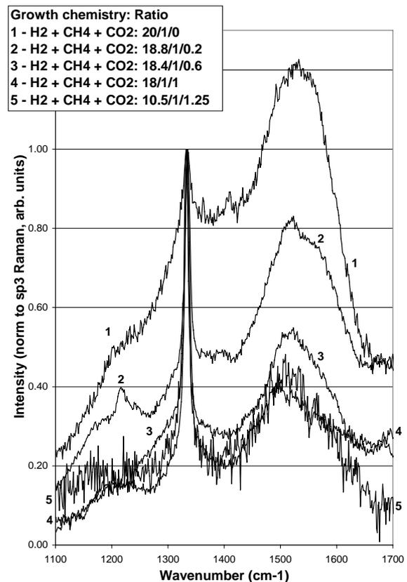
Fig. 3 Raman spectra of NCD films depending on  $\text{H}_2+\text{CH}_4+\text{CO}_2$  gas mixture.
