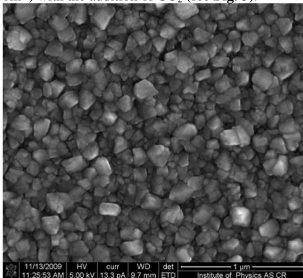
Fig. 2 SEM micrograph of prepared NCD film.
