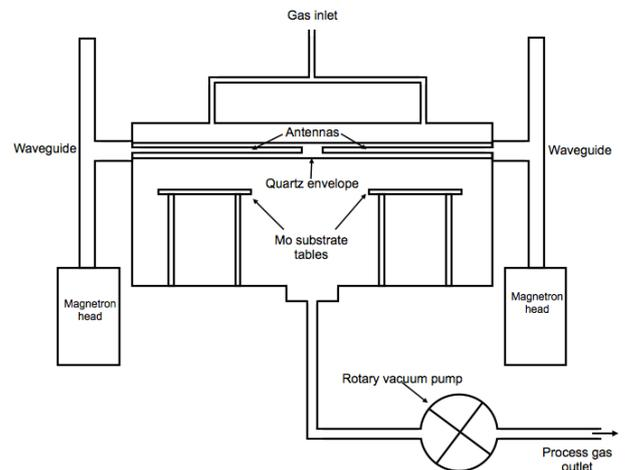
**Fig. 1** Photo and scheme of the non-commercial PELAMWCVD apparatus.
