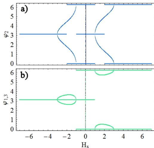
Fig.2 a) Angular evolution in response to the x-component of magnetic field  $H_x$  for the central particle b) The outer angles response to  $H_x$
