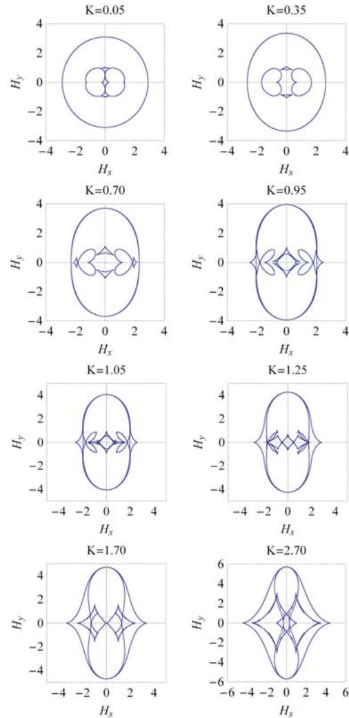
Fig. 3 For anisotropy values varied from  $K = 0.05$  to  $K = 2.70$  the critical lines of stability are shown for the applied magnetic field components  $H_x$  and  $H_y$ .
