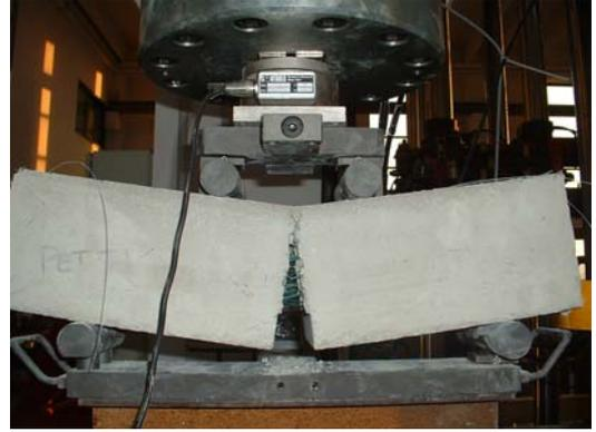
Fig. 1: Collapse configuration of a RPFRC/b specimen. The strong bridging effects played by PET fibers is visible.
