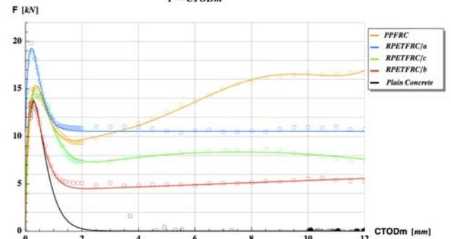
Fig. 2:  $F$ - $CTOD$  plots for different volumetric contents and types of recycled PET fibers.
