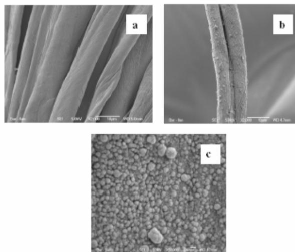
Figure 1. (a) HR-SEM images of pristine fibers, (b) fabrics coated with Ag nanoparticles at a low magnification, (c) fabrics coated with Ag nanoparticles at a high magnification
