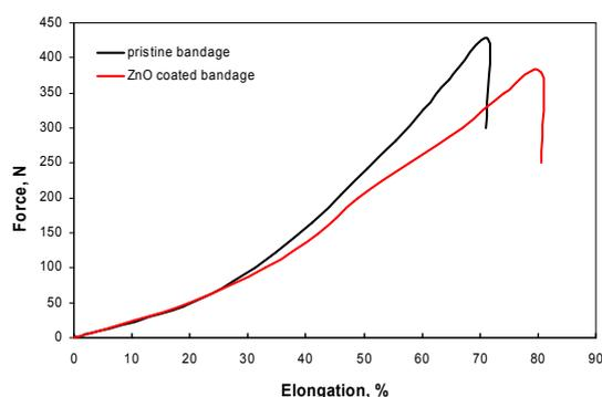
Figure 2. Mechanical properties of the cotton bandage before and after the deposition of ZnO nanoparticles.
