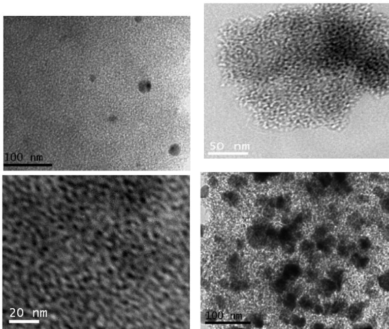
**Fig.4.** HRTEM micrographs of meso porous alumina and Ag nanoparticle incorporated alumina nanocomposites.
