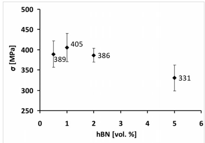
Fig. 2 Flexural strength of  $Al_2O_3$  - h.BN composite vs. hBN content
