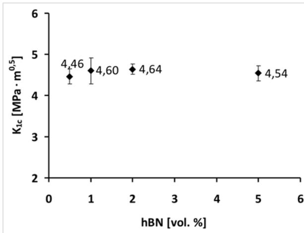
Fig. 1 Fracture toughness of  $Al_2O_3$  - h.BN composite vs. hBN content
