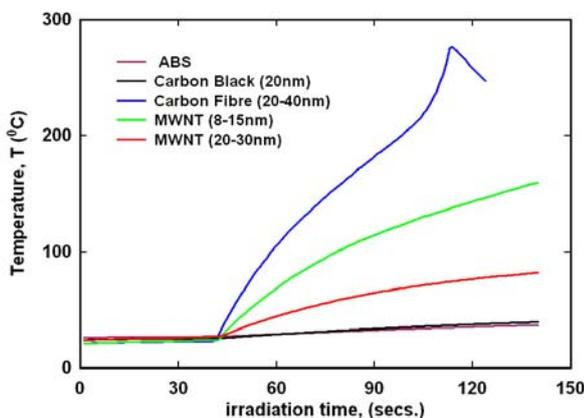
Figure 2: Measured temperature rise for 3% w/w carbon based nanofillers at 300 W irradiation power
