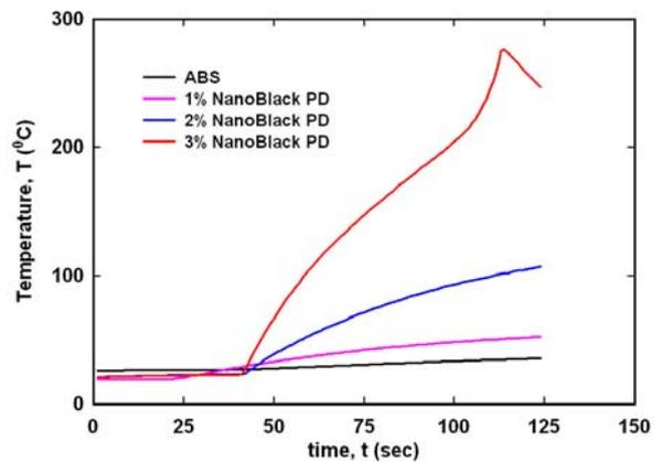
Figure 3: Measured temperature rise for varying levels of nano carbon fibres at 250W of microwave irradiation power.
