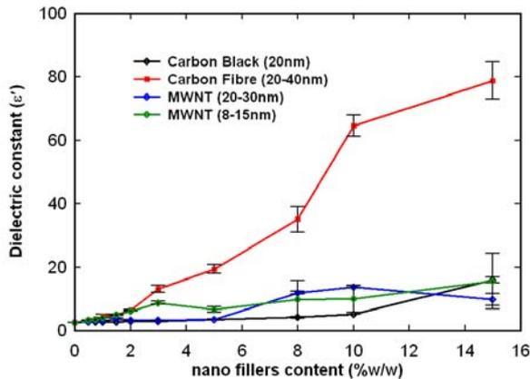
Figure 1: Dielectric constant for 3% w/w Carbon based nanofillers at 300 W microwave irradiation power.
