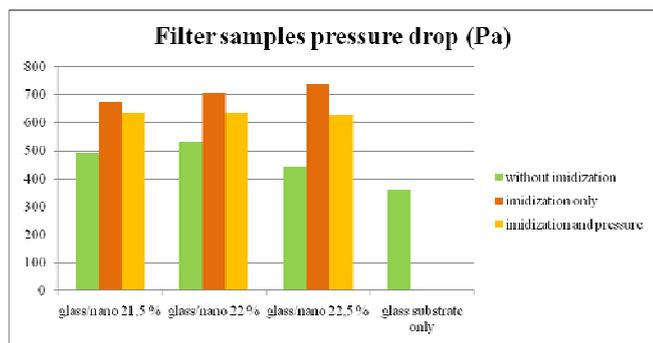
Fig. 2: Filter pressure drop of tested samples
