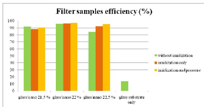
Fig. 1: Filter efficiency of tested samples
