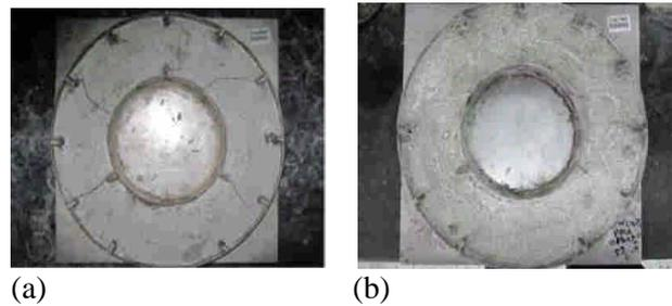
Fig. 4 The surface appearance of ring pastes with (a) 0% PAC, and (b) 0.1% PAC.
