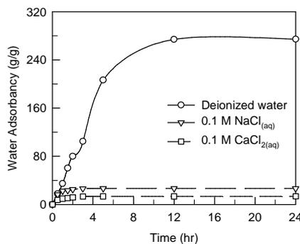
Fig. 1 Water absorbency of hydrogel versus time
