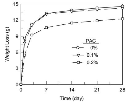
Fig. 2 The weight loss of mortars
