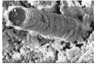
Figure 3. Photo of nano-silica coated glass fiber
