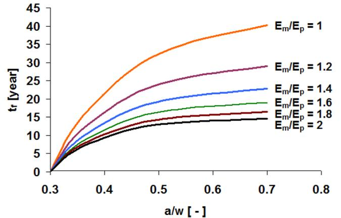
Fig.6. Residual lifetime of the pipe structure in the case of cracked inner protective layer for different ratio between Young modulus of the main pipe ( $E_m$ ) and protective layer ( $E_p$ ).
