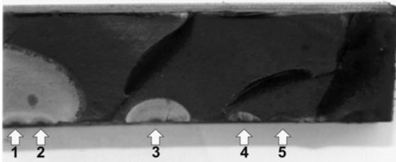
Fig.1. Multiple fracture initiation sites on the inner wall of a failed HDPE tube. The final fracture surface is fully fragile. A length scale is established by the thickness of the tube, which is 40 mm [2].
