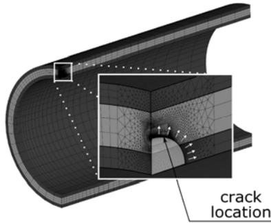
Fig.4. Finite element model of the internally pressured pipe with crack in the main layer from HDPE material
