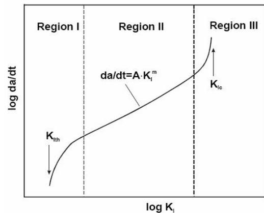
Fig.3. Scheme of creep crack growth rate curve [3].
