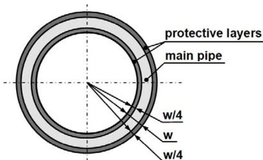
Fig.2. Scheme of three layer pipe studied in the article.
