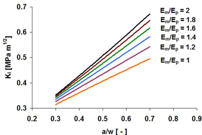
Fig.5. Stress intensity factors obtained for different ratio between Young modulus of the main pipe ( $E_m$ ) and protective layer ( $E_p$ ).
