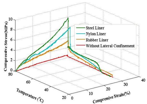
Fig.1 Programming of the foam with various confinements
