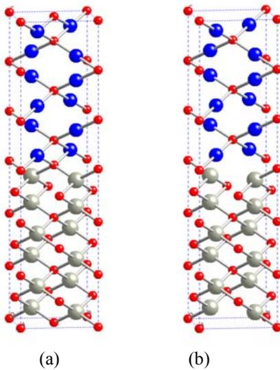
Fig. 1 Supercells used for calculating  $\Delta E_v$ , consisting of Cu<sub>2</sub>O and zincblende ZnO. The small filled circles are O, the medium dark circles Cu, and the gray large circles Zn. The interface atomic layer is ZnO-like in (a) and Cu<sub>2</sub>O-like in (b).
