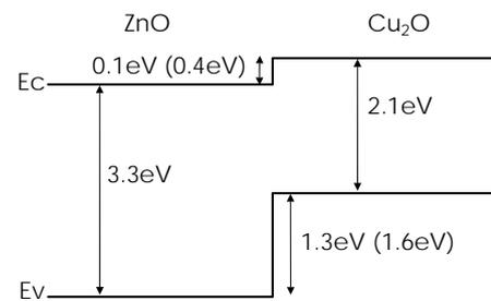
Fig. 4 Schematic of the predicted band alignment for ZnO/Cu<sub>2</sub>O.
