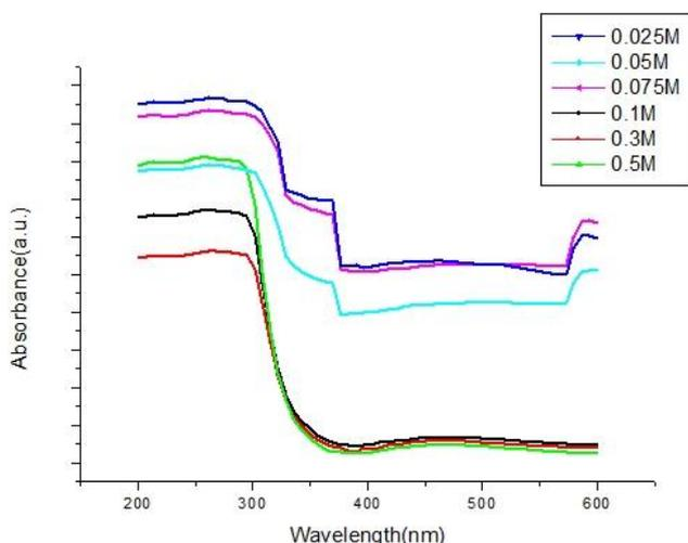
**Fig. 2 UV-Vis spectroscopy of the ZnO nanorods grown on ITO glass with different concentration of precursors.**
