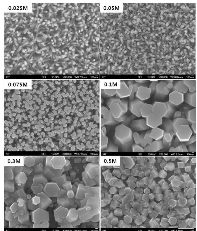
Fig. 1 SEM images of ZnO nanorods grown on ITO glass with different concentration of precursors.
