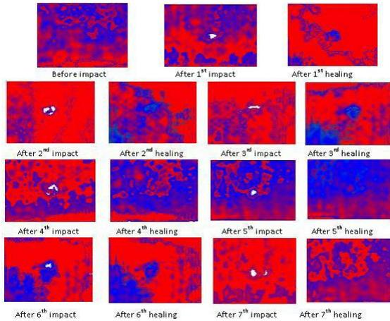
Fig. 5 C-scan images of the sandwich panels after each impact and healing cycle
