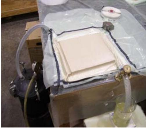
Fig.1 Vacuum Assisted Resin Infusion Method
