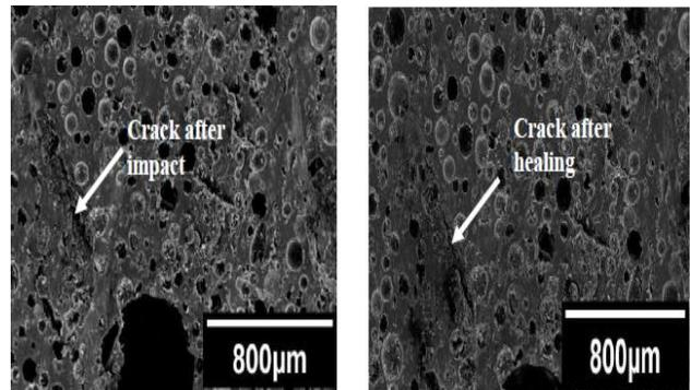
Fig.6 SEM pictures showing the effect of healing on the microcrack
