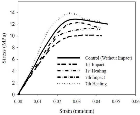
Fig.3. Typical CAI stress versus strain plots for various impact and healing cycles
