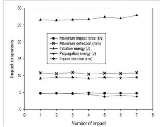
Fig.2 Impact response of the smart foam cored sandwich panels under multiple impacts
