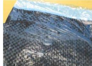
Fig.1(a) Woven CFRP prepreg.
