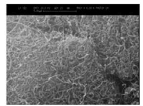
Fig.1(b) SEM of dry CNT.
