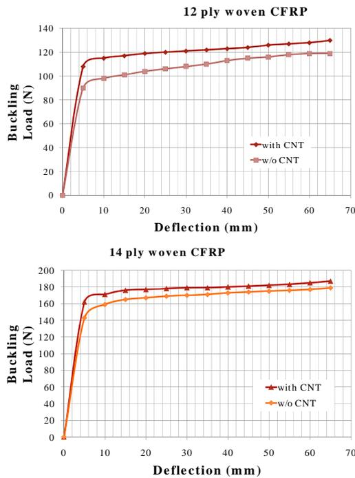
Fig. 4 Buckling behaviour of woven CFRP laminates.
