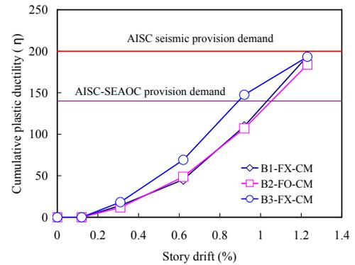
Fig. 3 Ductility capacity ( $\eta$ )
