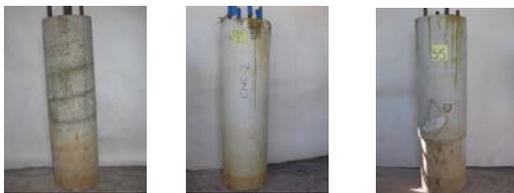
**Figure 1a. Unwrapped Specimen**
