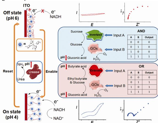
**Fig. 4.** Logic operations **AND/OR** performed by the enzyme-based systems resulting in the **ON** and **OFF** states of the bioelectrocatalytic interface followed by the **Reset** function to complete the reversible cycle.
