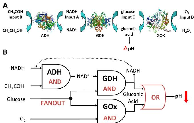
**Fig. 1.** (A) The multi-gate / multi-signal processing enzyme logic system producing *in situ* pH changes as the output signal. (B) The equivalent logic circuitry for the biocatalytic cascade.
