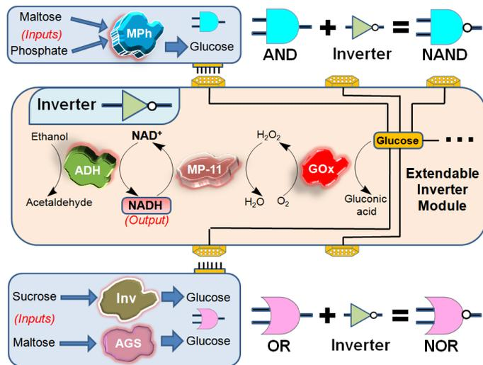
**Fig. 3.** Modular design of the enzyme-based NAND and NOR gates.
