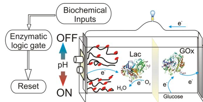
**Fig. 5.** The switchable biofuel cell controlled by pH changes produced *in situ* by the enzyme logic systems processing biochemical inputs.
