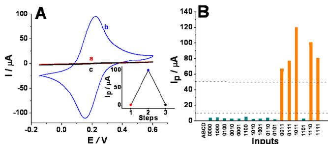
**Fig. 2.** (A) Cyclic voltammograms obtained for a signal-responsive switchable electrode controlled by the enzyme logic network: a) initial OFF state, b) ON state enabled by the input combinations, c) *in situ* reset to the OFF state. Inset: reversible current changes upon switching the electrode ON-OFF. (B) Anodic peak currents,  $I_p$ , for the 16 possible input combinations.
