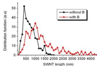
**Fig. 1. Length distribution of SWNT with and without magnetic field.**
