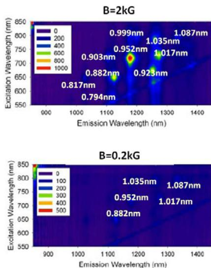
Fig.3. Photoluminescence (PL) characterization of the SWNT sample with magnetic field as a parameter.
