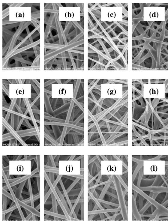
Figure 1. Morphology of PVDF-PU nonwoven webs with 10 %wt concentration of the core solution at a volume feed rate of (a) 0.06, (b) 0.1, (c) 0.5, and (d) 1.0 ml/h; with 15 %wt concentration of the core solution at a volume feed rate of (e) 0.06, (f) 0.1, (g) 0.5, and (h) 1.0 ml/h; and with 20 %wt concentration of the core solution at a volume feed rate of (i) 0.06, (j) 0.1, (k) 0.5, and (l) 1.0 ml/h.
