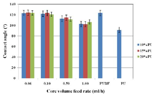
Figure 2. Water contact angle of the nonwoven webs of polyurethane (PU) (core) with different concentrations (10, 15, and 20 wt%) and polyvinylidene fluoride (PVDF) (sheath) with a fixed concentration of 20 wt%.
