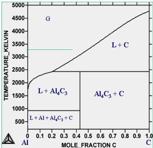
Figure 1 Phase diagram of Al-C system determined by Calphad modeling.
