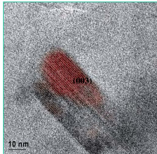
Figure 3 HR-TEM image showing presence of rod-shaped  $\text{Al}_4\text{C}_3$  precipitates in the nanocomposite sample.
