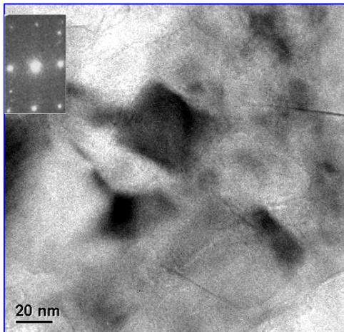
Figure 2 Micrograph showing morphology of nanosized diamond particles in the Al matrix nanocomposite specimen, inset SADP, Z=[123]Diamond.
