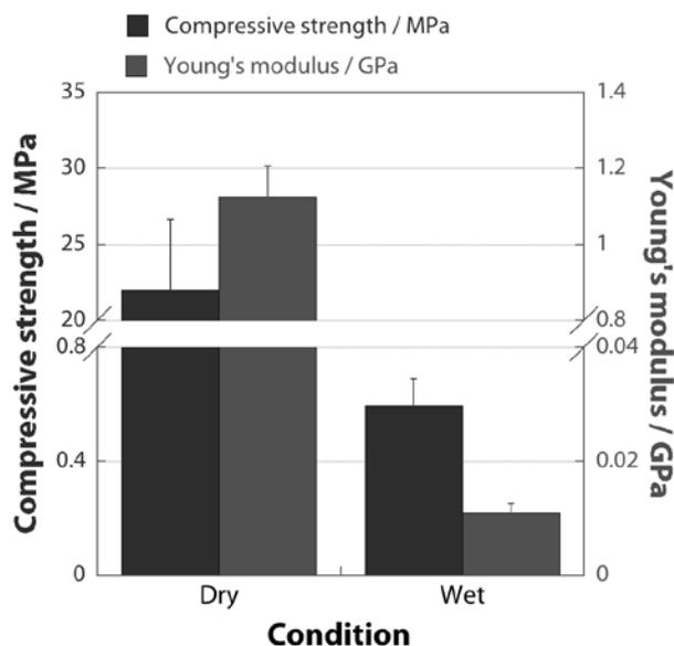
Fig. 2. Mechanical properties of core-shell type HAp/Col artificial bone.
