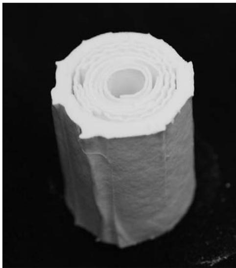
Fig. 1. Core-shell type HAp/Col artificial bone.
