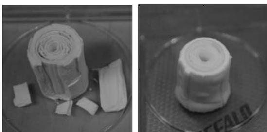
Fig. 3. Core-shell type HAp/Col artificial bone in dry (left) and wet (right) condition after compressive strength test.
