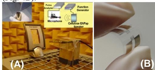
Fig. 4. EAPap based acoustic devices (A) paper speaker (B) SAW device.
