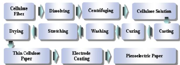
Fig. 1. Cellulose EAPap fabrication process.
