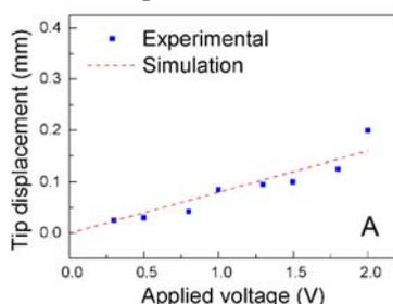
Fig. 3. Comparison of bending displacement from simulation model and the experimental results.
