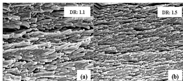
Fig. 2. SEM cross-sectional images of stretched cellulose film along with drawing ratio.
