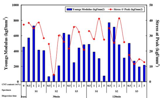
Fig. 2 Tensile properties of the PU/MWNT film according to the dispersion condition.
