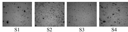
Fig. 4 Photograph of surface of the PU/MWNT film. (dispersion time 120min., contents of MWNT 1wt%)
