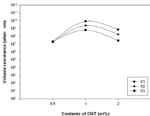
Fig. 3 Resistance values of the PU/MWNT film according to the dispersion condition.
