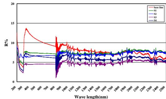
Fig. 1 Reflection rate of the PU/MWNT film according to the MWNT types. (dispersion time 30min., contents of MWNT 1wt%)
