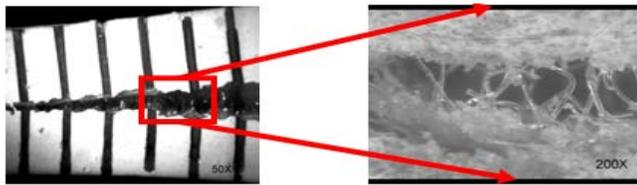
Fig. 3 Toughening mechanism of Z-fiber reinforced laminar composites.
