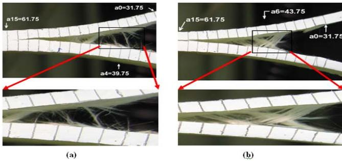
Fig. 2 Fiber bridging (a) and yarn bridging (b) in 3-D composites.
