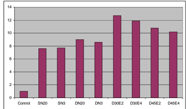
Fig. 4 Comparison of Mode I fracture toughness for 3-D braided and Z-microfiber reinforced composites.
