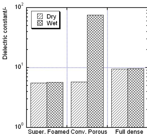
Fig.2 Dielectric constant of alumina based ceramics with dry and wet conditions
