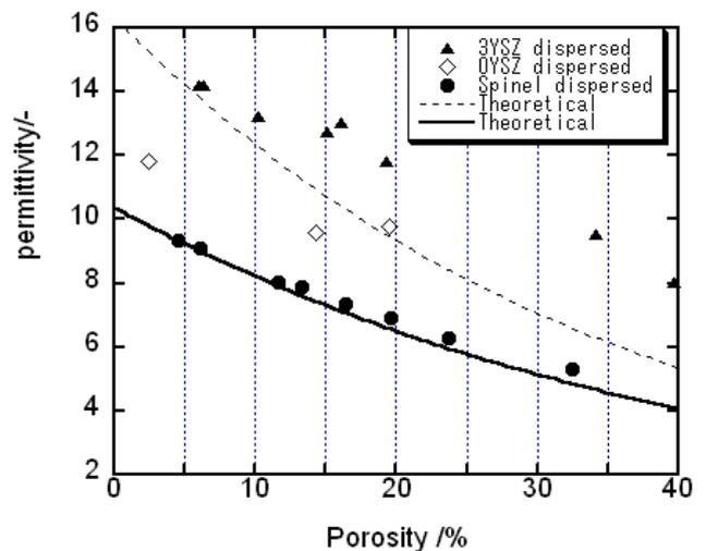
Fig.1 Porosity dependence of dielectric constant for superplastically foamed ceramics dispersed with spinel or 0YSZ.
