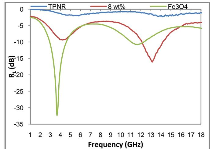
Fig. 3. Absorption characteristics of the TPNR, Fe<sub>3</sub>O<sub>4</sub> and nanocomposites
