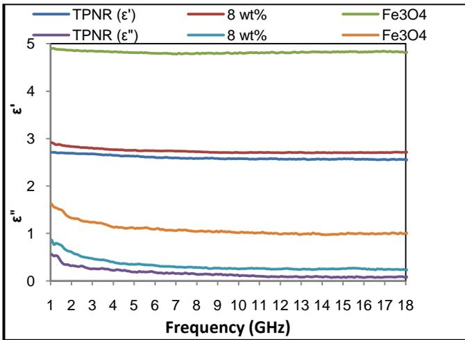
Fig . 1. Permittivity spectra of the TPNR, Fe<sub>3</sub>O<sub>4</sub> and nanocomposites.
