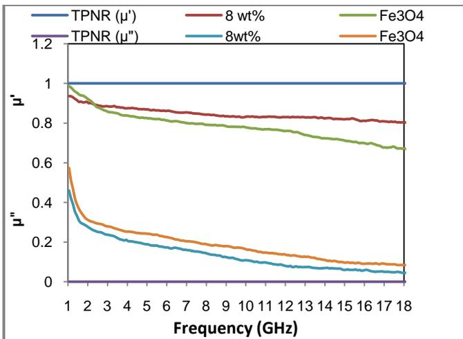
Fig. 2. Permeability spectra of the TPNR, Fe<sub>3</sub>O<sub>4</sub> and nanocomposites.
