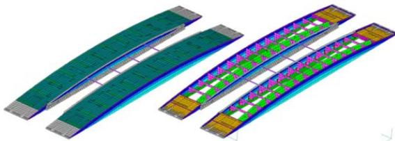
Fig 6 Composite Army Bridge internal structure
