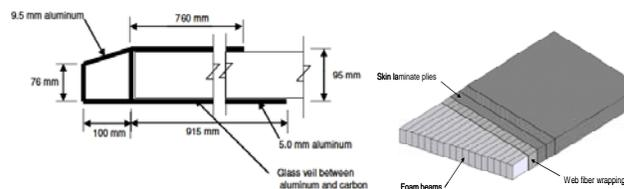
Fig 3 Illustration of end-cap and trackway cut away.
