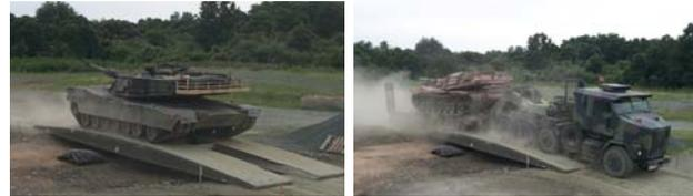
Fig 7 CAB field testing: M1A1 and HET.
