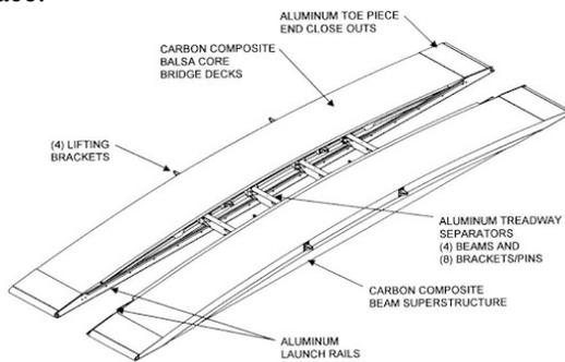
Fig 5 Composite Army Bridge (CAB) design features.
