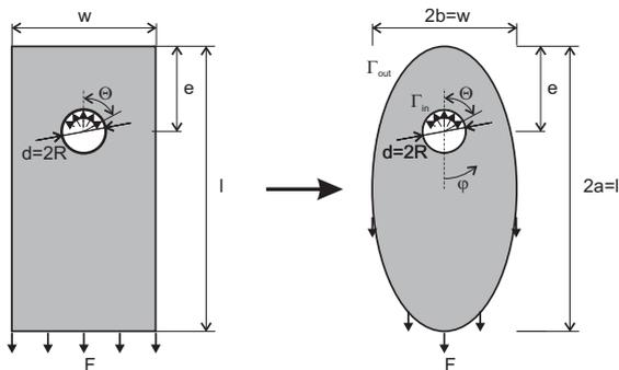
Fig. 1 The geometry of the specimen and its approximation
