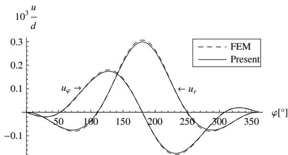
Fig. 3 Radial  $u_r$  and tangential  $u_\varphi$  displacement on notch border for  $[\pm 45^\circ]_s$ ,  $w/d=3$
