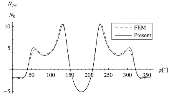
Fig. 4 Tangential section force  $N_{\varphi\varphi}$  on notch border for  $[\pm 45^\circ]_s$ ,  $w/d=3$
