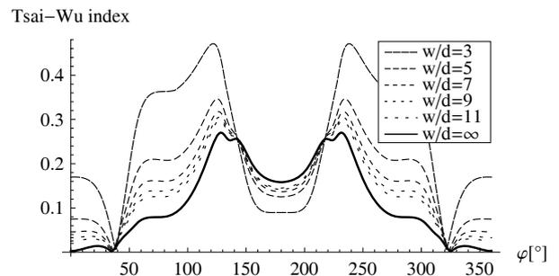
Fig. 5 Maximal Tsai-Wu index on the notch border for  $[\pm 45^\circ]_s$  for various values of the  $w/d$  ratio including the infinite plate
