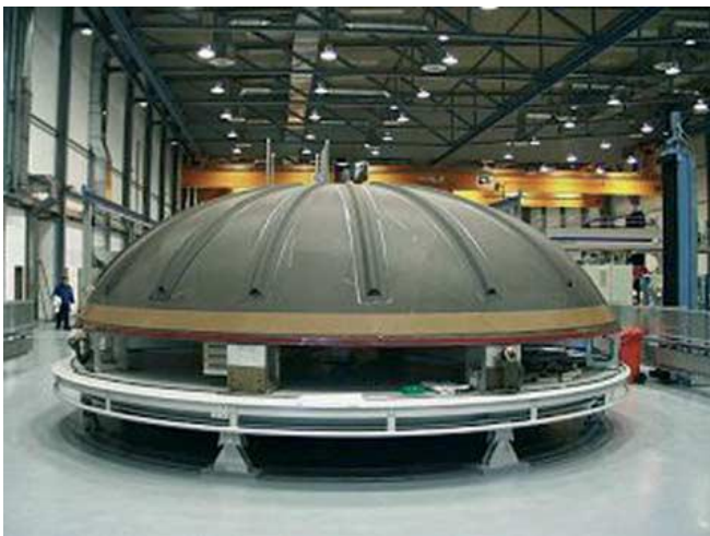
Fig. 1. The Airbus A380 rear pressure bulk head, made of carbon NCFs [Saertex]
