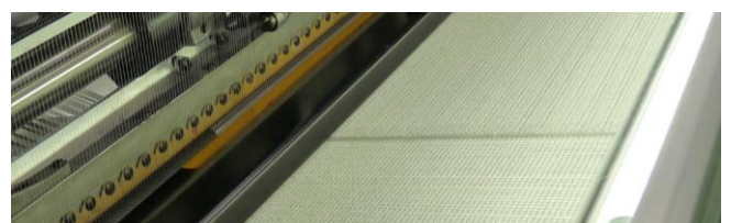
Fig. 3: Production of a 24 layer NCF with variation in thickness
