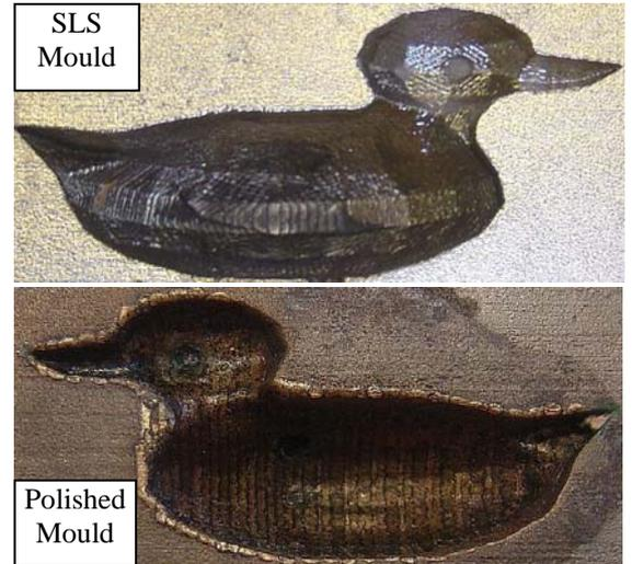
Fig. 5. SLS mould (top) and laser polished (bottom)
