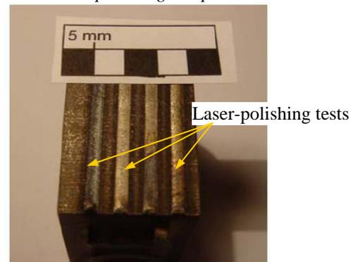
Fig. 1. Simple line polishing test part
