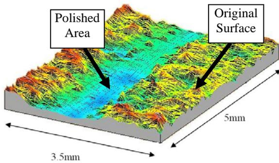
Fig. 3. Topography of laser polishing test
